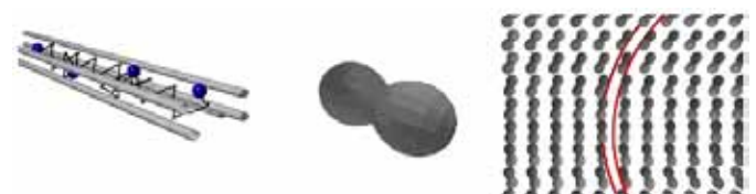
Figure 2 In regions with closely packed fiber bundles the water diffusion is found to be anisotropic (left image). The water self diffusion characteristics can be described by a tensor (middle image). Following the main axis in each tensor in a stepwise fashion from tensor to tensor forms the basis of fiber tracking (right image).
