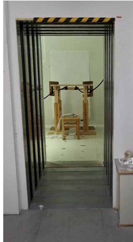
Figure 3 James Lubell visited the Physikalisch-Technische Bundesanstalt in Berlin with our OPMs to make use of their BMSR2 facility, the most magnetically quiet place on Earth. This allowed him to investigate the upper frequency limits of OPMs for measuring human neural activity in a virtually noise-free environment.
