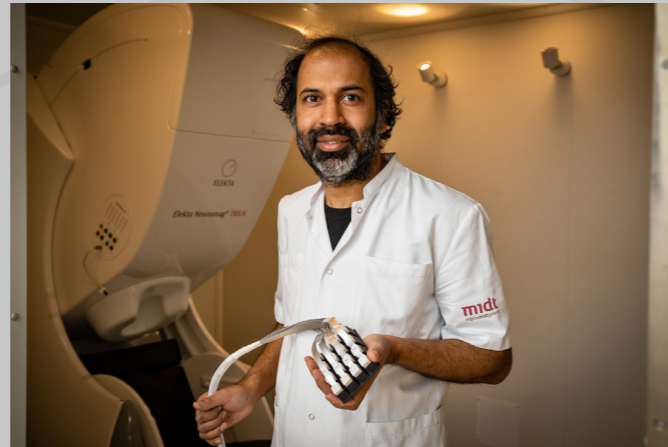
Figure 1 In early 2020, we received a starter set of 16 OPMs from FieldLine Inc. (Boulder, Colorado) for measuring MEG and other biomagnetic signals from the human body.
